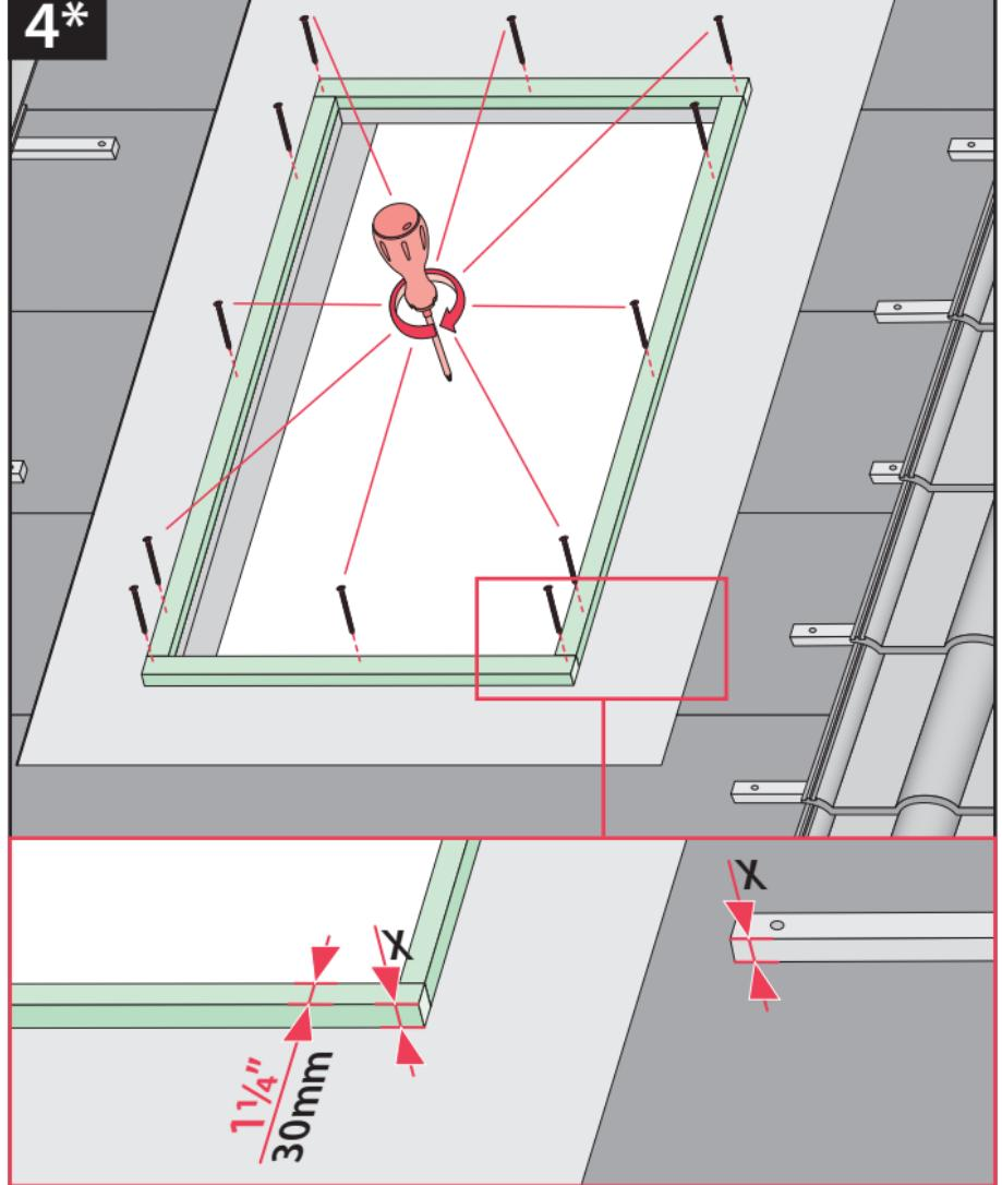
**US** Place 1 1/4" (30mm) wide battens around the rough opening. Battens should be of the same thickness as battens used for roofing material.
