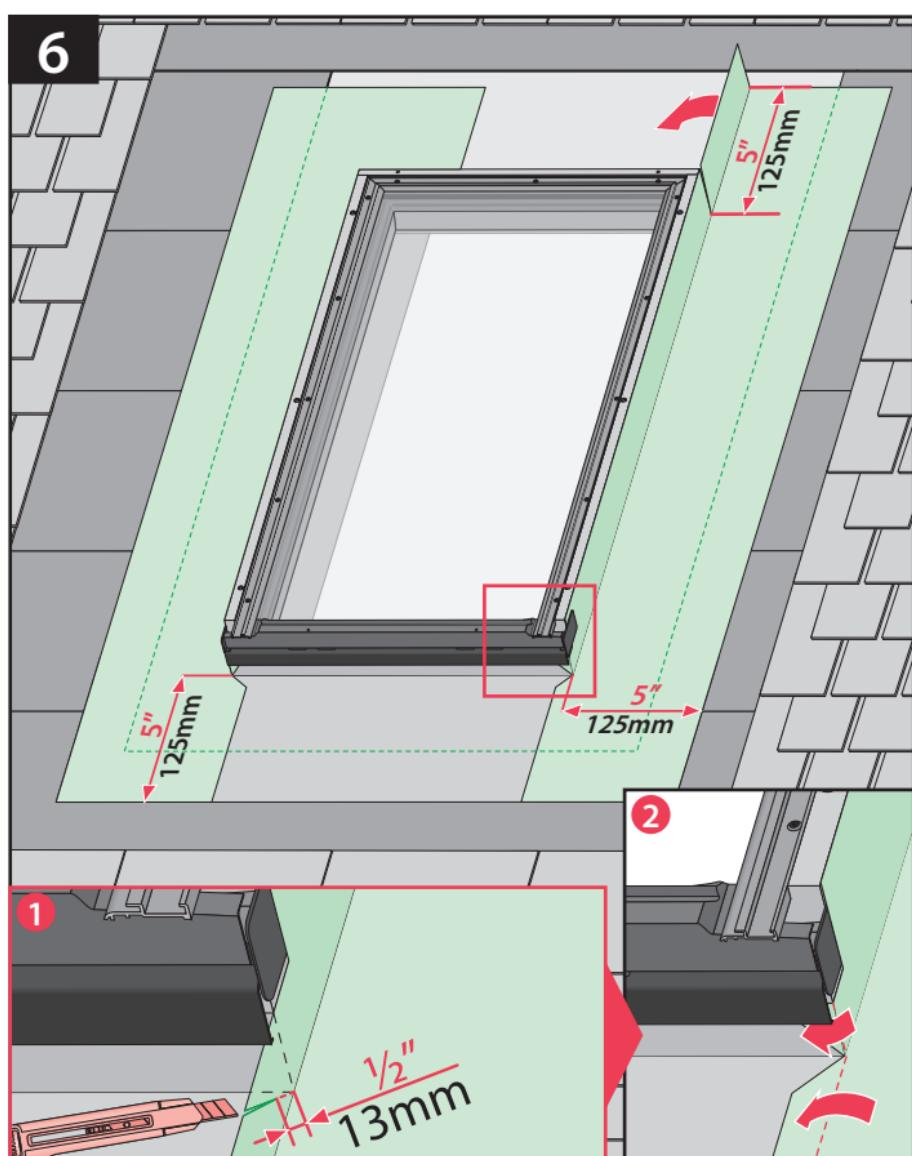
**US** Wrap the sides and corners of the frame overlapping 3" (75mm) over the underlayment.
