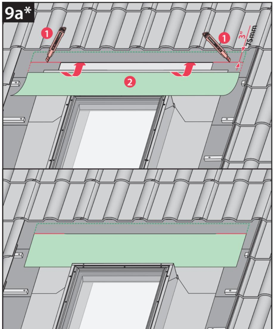
**US** To ensure proper water drainage, interweave the skylight's underlayment with the existing roofunderlayment (retrofit).
