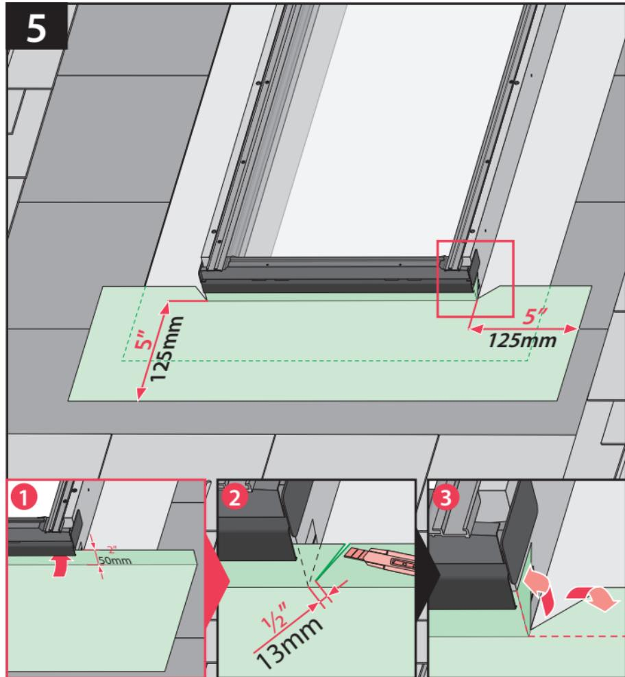
**US** For complete waterproofing, apply self-adhesive roofing underlayment also called Ice & Water Guard. Wrap the bottom frame with corners first. Keep minimum 3" (75mm)overlap with existing roofing underlayment.
