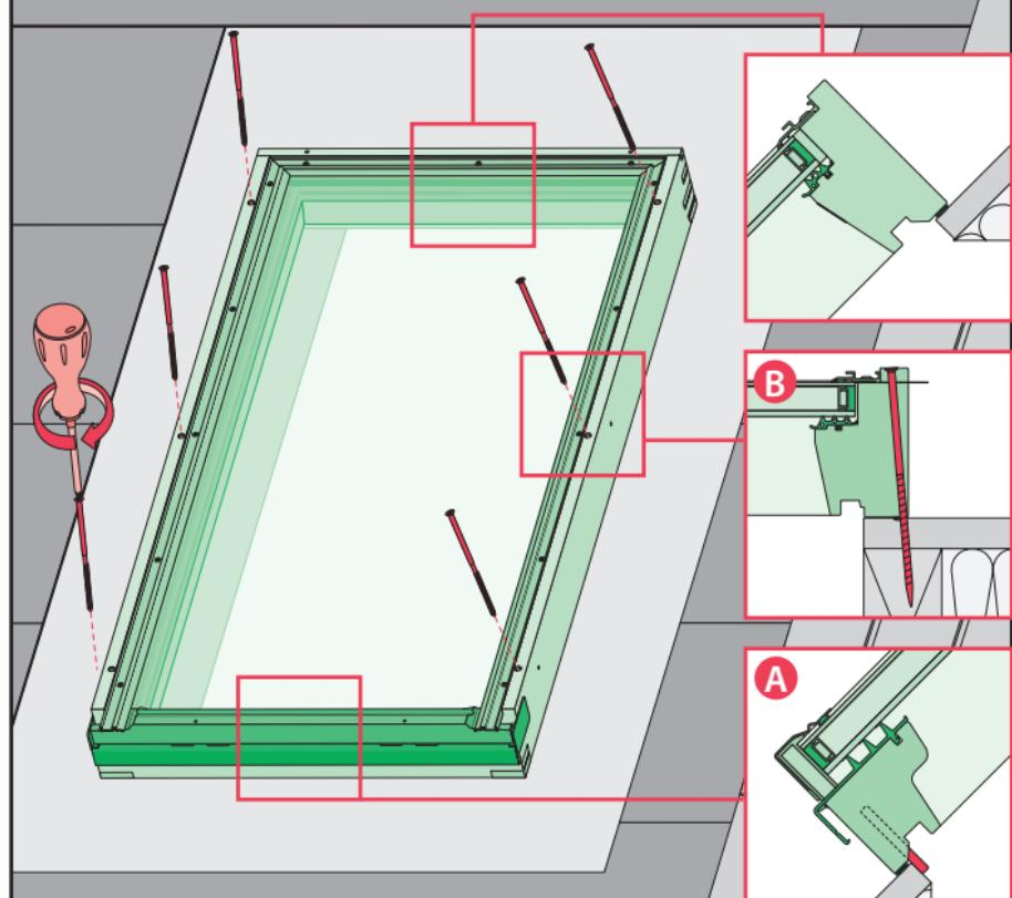
**US** Place the skylight's frame over the rough opening with the pins (A) resting on a bottom edge of the opening. Screw in provided screws (B) through the pre-drilled holes to secure the frame in place. Make sure the diagonals are equal.
