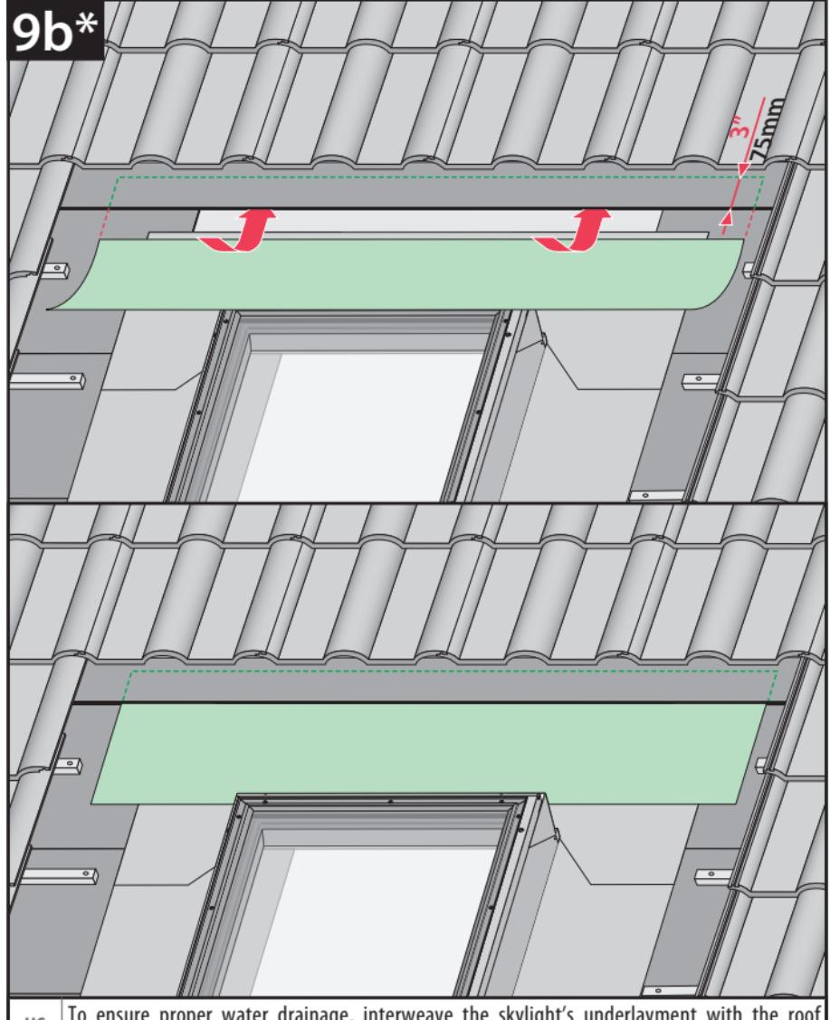
**US** To ensure proper water drainage, interweave the skylight's underlayment with the roof underlayment (new construction).
