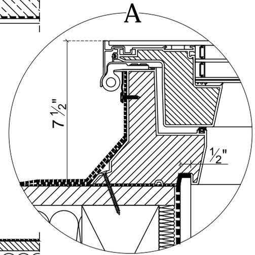
735-DRF DU6 Flat Roof Window, manually opened, Flat, glazing unit DU6
