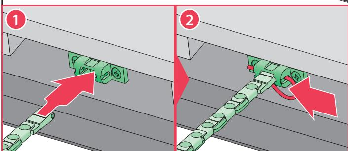
**US** Place the end of the chain into the holder on the skylight's sash and block it with the pin.
