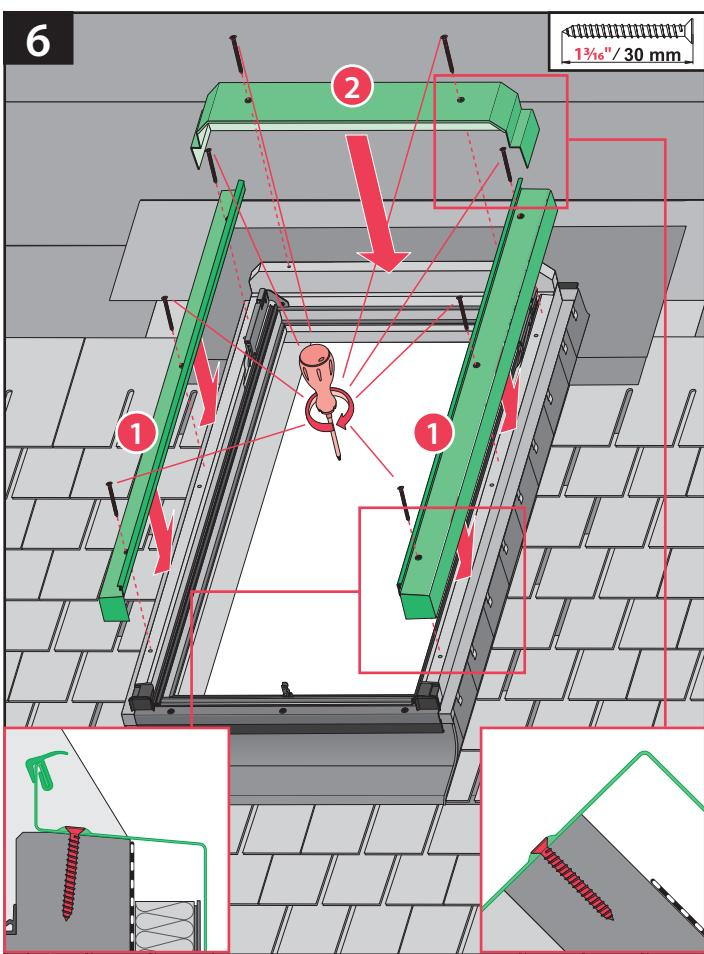
**US** Replace side and top covering profiles of the frame. Secure them with the screws.
