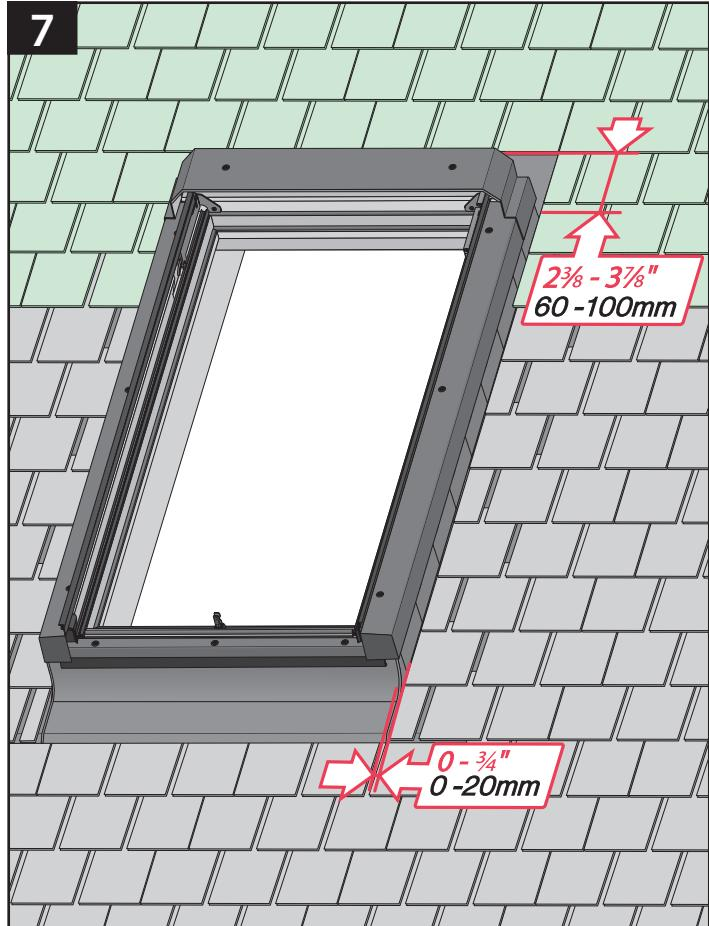
**US** Finish the roofing material on sides and above the skylight.
