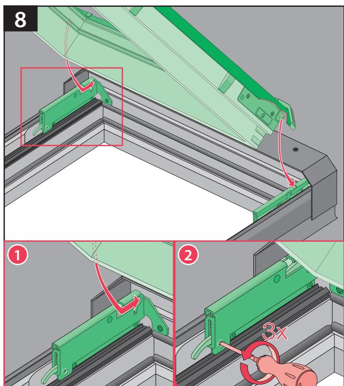
**US** Insert the sash according to the direction of the arrow, allowing the side-prong to slide into the hinge slider. Unscrew the locking screw (3 turns) blocking the hinge.
