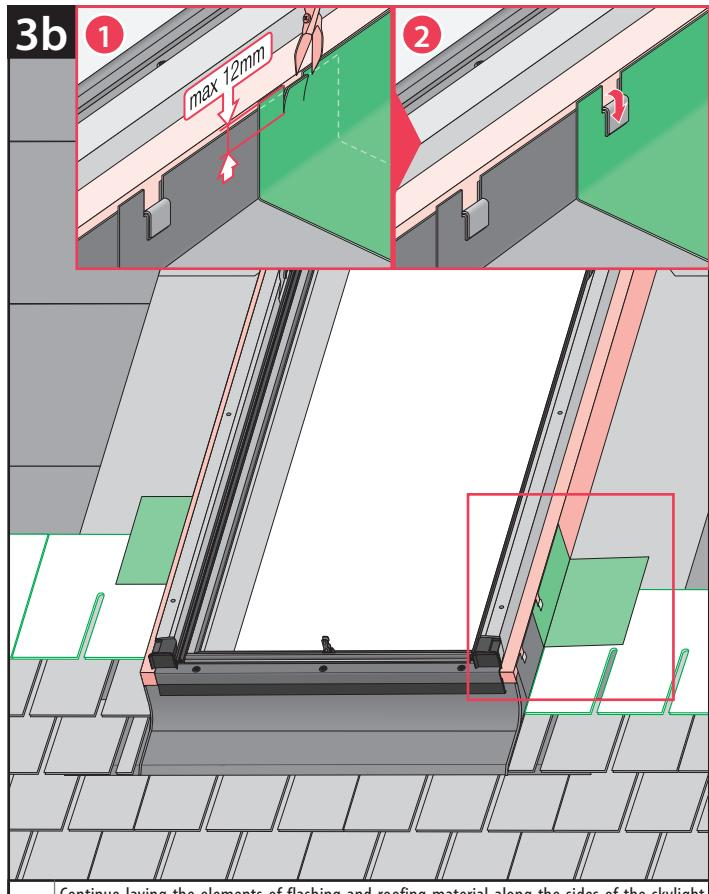
**US** Continue laying the elements of flashing and roofing material along the sides of the skylight upwards.
