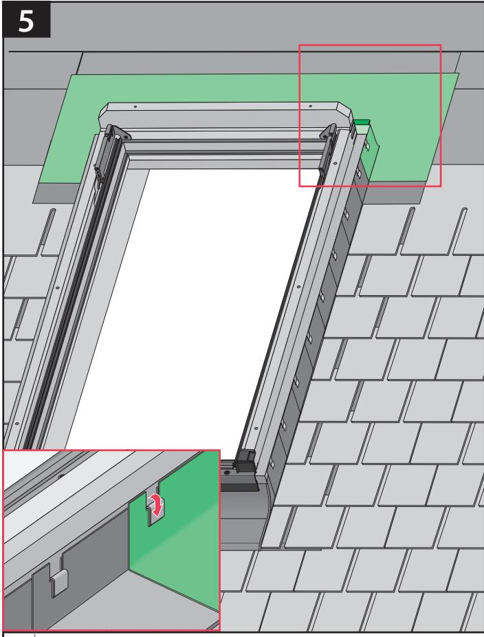
**US** Place the upper part of the flashing and connect with the side elements as shown in the picture.
