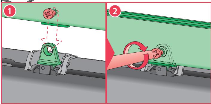
**US** Close the sash and secure the end of the chain with the screw.
