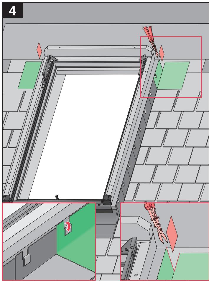
**US** If necessary, cut the last part accordingly.
