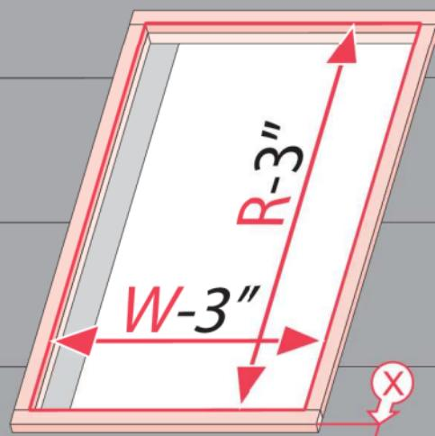
**US** Prepare the rough opening in the roof in the dimensions of W-3" i R-3" (dimensions W and R are given in a table on page 2). Place wooden battens around the opening. Battens should be of the same thickness as battens used for roofing material.
