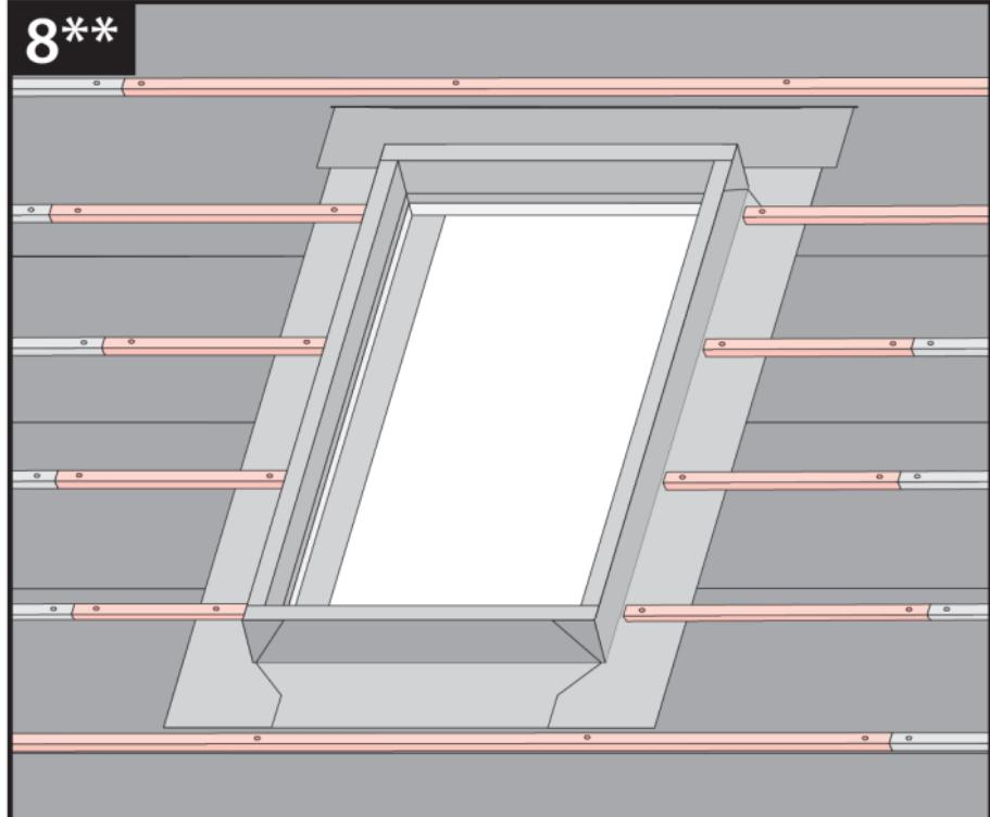
**US** Replace the battens around the rough opening.
