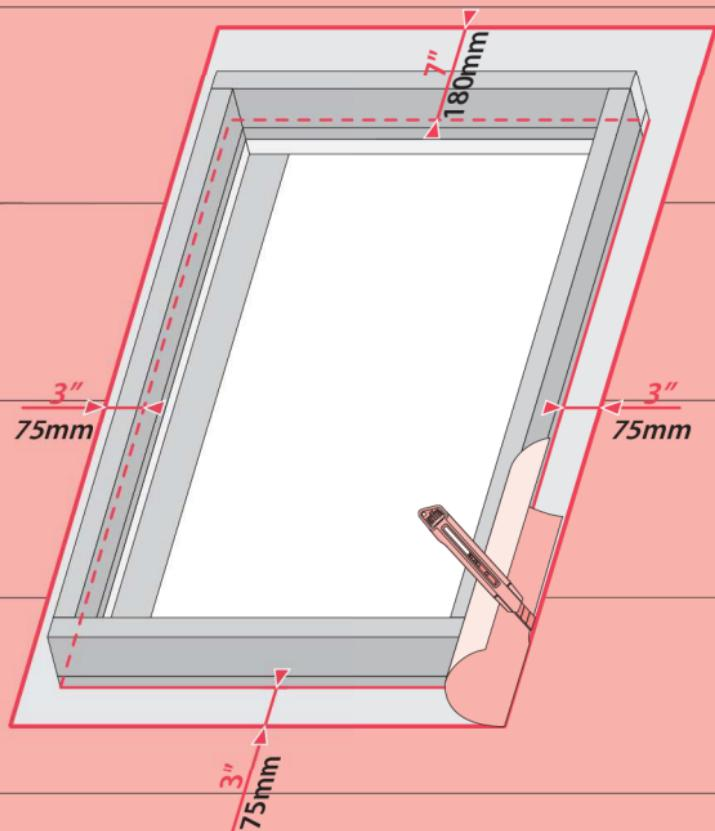
US Remove existing roofing underlayment around the opening.
