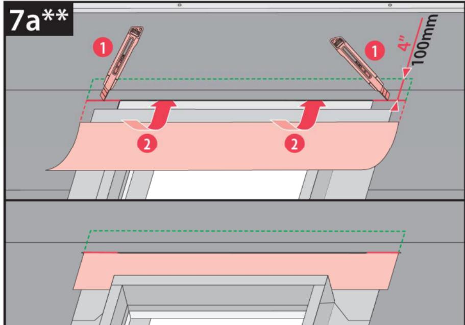
**US** To ensure proper water drainage, interweave the skylight's underlayment with the existing roof underlayment (retrofit).
