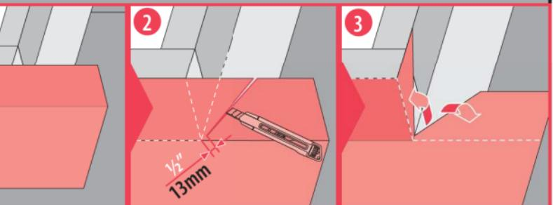
US For complete waterproofing, apply self-adhesive underlayment at the bottom of the curb.
