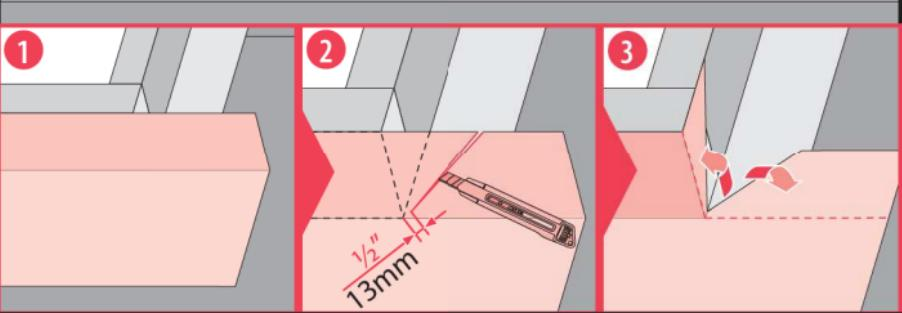
US For complete waterproofing, apply self-adhesive underlayment at the bottom of the curb.
