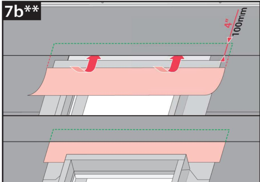
**US** To ensure proper water drainage, interweave the skylight's underlayment with the new roof underlayment (new construction).
