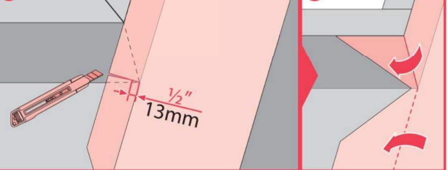
US Apply self-adhesive underlayment on the sides of the curb.
