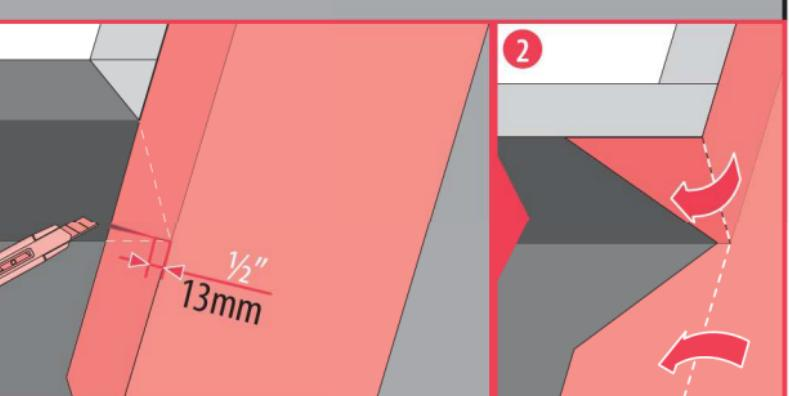
US Apply self-adhesive underlayment on the sides of the curb.
