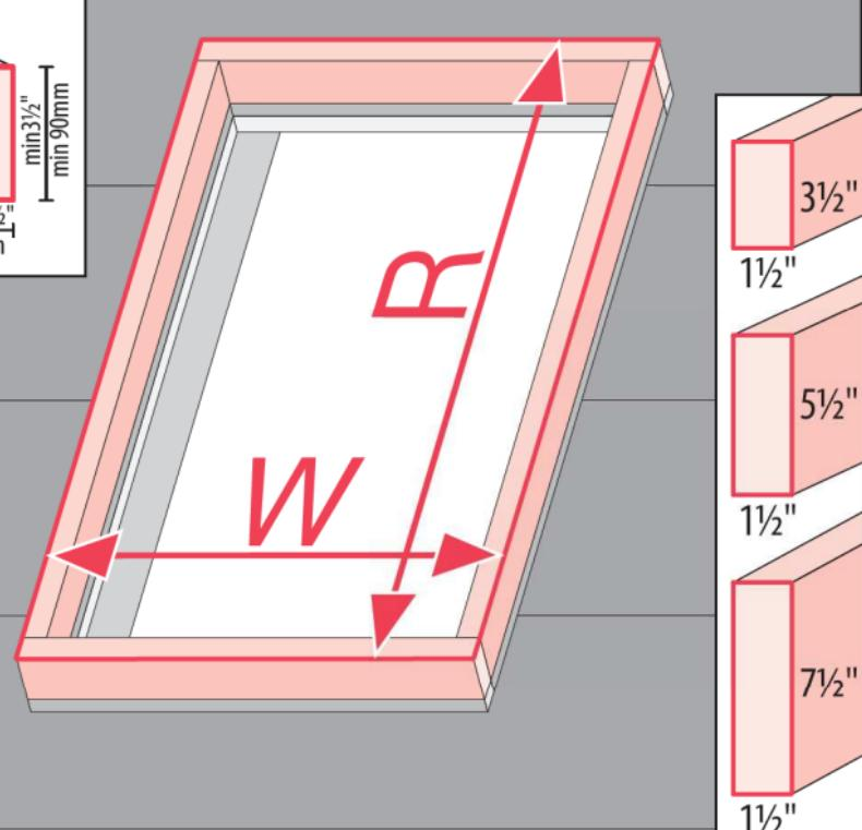
**US** Build a curb around the rough opening using a standard 2x4, 2x6 or 2x8 lumber.
